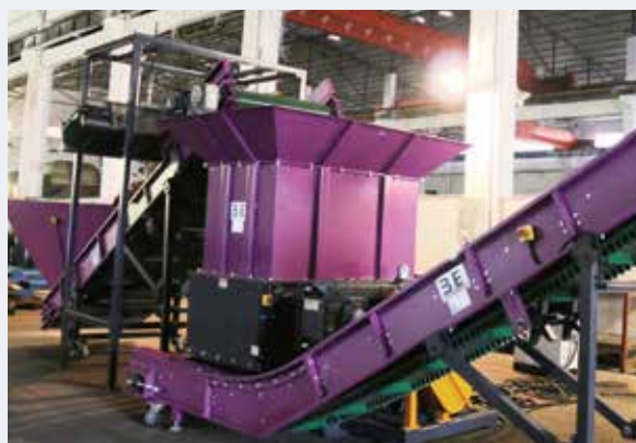
单轴撕碎机WTF40120配磁选生产线 Single shaft shredder WTF40120 with magnetic separation
