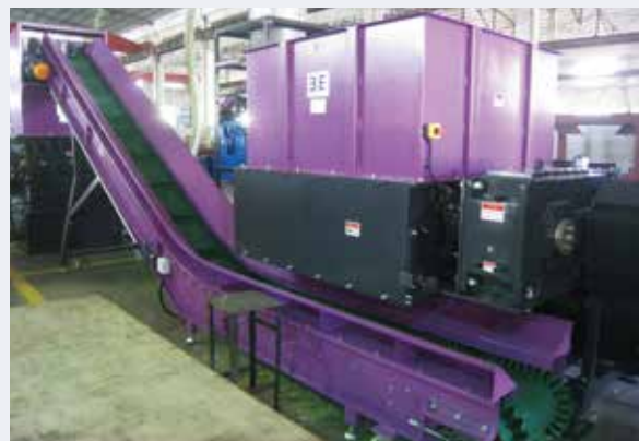
单轴撕碎机WT40150+破碎机PC52120生产线 Single shaft shredder WT40150 with Granulator PC52120
