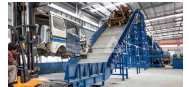
报废汽车车身回收线 Car shell crushing & recycling line 10000kg/h
