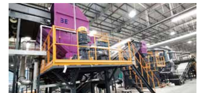
冰箱破碎线 Refrigerator recycling line 100 units/hour
